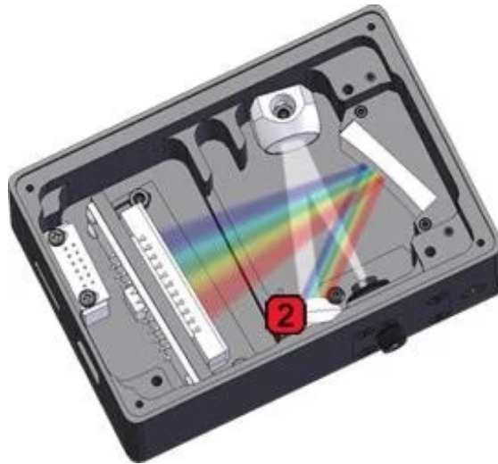
Figure 5: A diffraction spectrometer diffracts a beam of collimated light.
