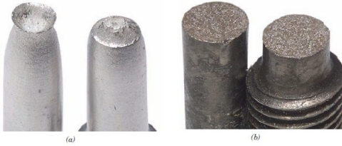
Fig. 14. The difference between a flat, brittle fracture perpendicular to applied force, versus the cup and cone relic of a ductile fracture.
