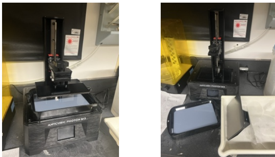
Fig. 10. (left) A view of the lab's Anycubic Photon M3 resin printer. (right) A view of the printer with resin tray and build plate removed, revealing the UV screen under the tray.
