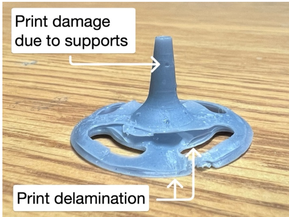
Fig. 14. An iteration of the print showing severe delamination of the base, as well as physical damage to the print from removal of supports. Note that we attempted printing the nozzle upside-down (with the nozzle exit towards the base) to avoid this problem, but encountered incorrigible asymmetries in the final print.
