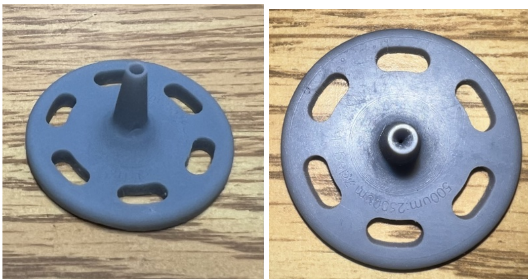
Fig. 15. A top and side view of the final nozzle, with clear throat.
