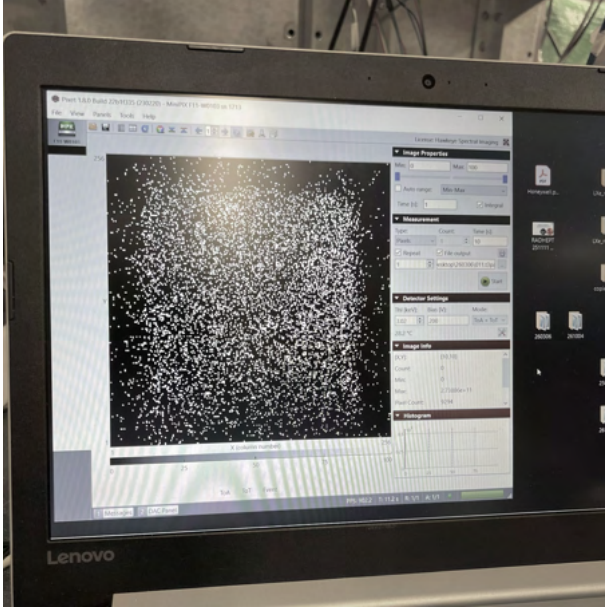
Fig. 11. Electrical interference produced by the outgassing breakdown resulted in static-like noise on the MiniPIX radiation counter, inhibiting analysis of generated particles.
